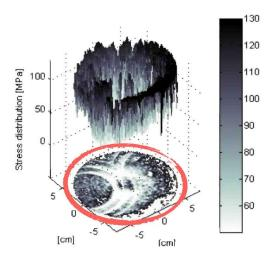
(1) Yen-kuei Chang., 2007, "The investigation of the compressive stress deviation of concrete cylinders under different capping methods using the pressure sensitive films." p74-97
