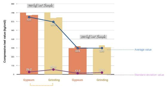
They had greater effects on the strengths of cylinders made of high-strength concrete compared with cylinders of low-strength concrete<sup>(3)</sup>.
