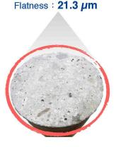
The concrete surface is treated by the grinding knife. It is difficult to get a completely smooth surface. Without the periodic maintenance, the knife has a high possibility to be damaged causing a poor end surface.
