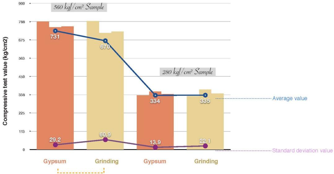
They had greater effects on the strengths of cylinders made of high-strength concrete compared with cylinders of low-strength concrete(3).
