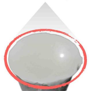
The completely smooth surface comes from the flowing gypsum slurry and thick glass plate. After being covered by the glass, the gypsum surface will be flat just like glass similar to a mirror.
