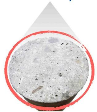
The concrete surface is treated by the grinding knife. It is difficult to get a completely smooth surface. Without the periodic maintenance, the knife has a high possibility to be damaged causing a poor end surface.
